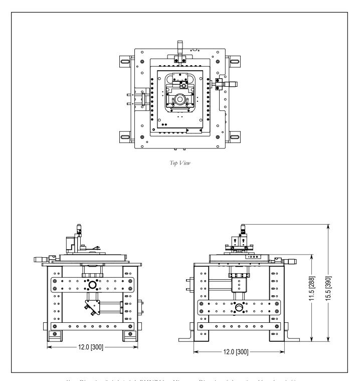
Above: Dimensions (in inches) of the RM21  $^{\text{\tiny TM}}$  Versa Microscope. Dimensions of the metric model are shown in [].
